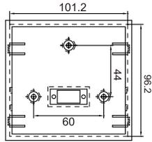
钣金安装开孔尺寸: 101.2mm\*96.2mm
