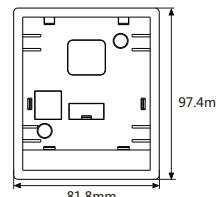
钣金安装开孔尺寸: 97.4mm\*81.8mm
